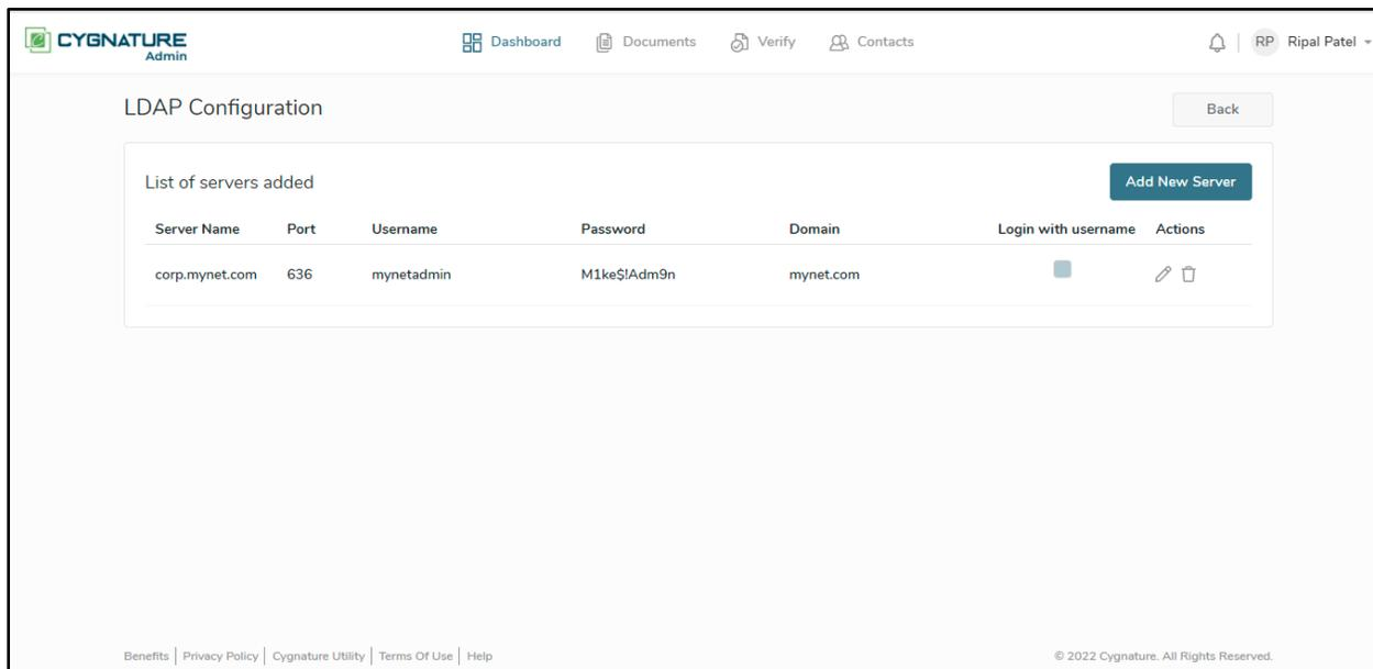
Click on Add New Server to set multiple LDAP servers to pass LDAP login. Add the required LDAP details and test LDAP connection if set successful
